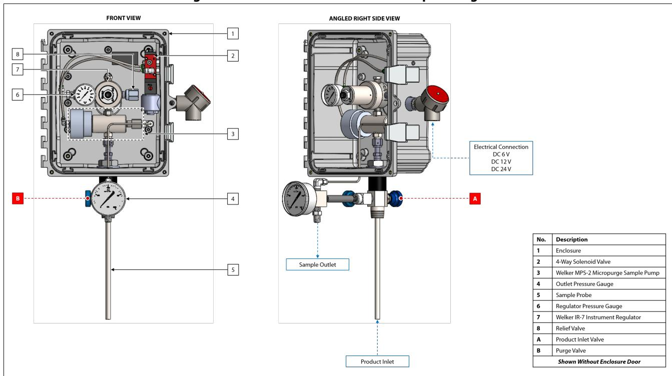
**Figure 2: Essentials™ Gas Sampler With Optional Welker 6Tc Timer/Controller**
