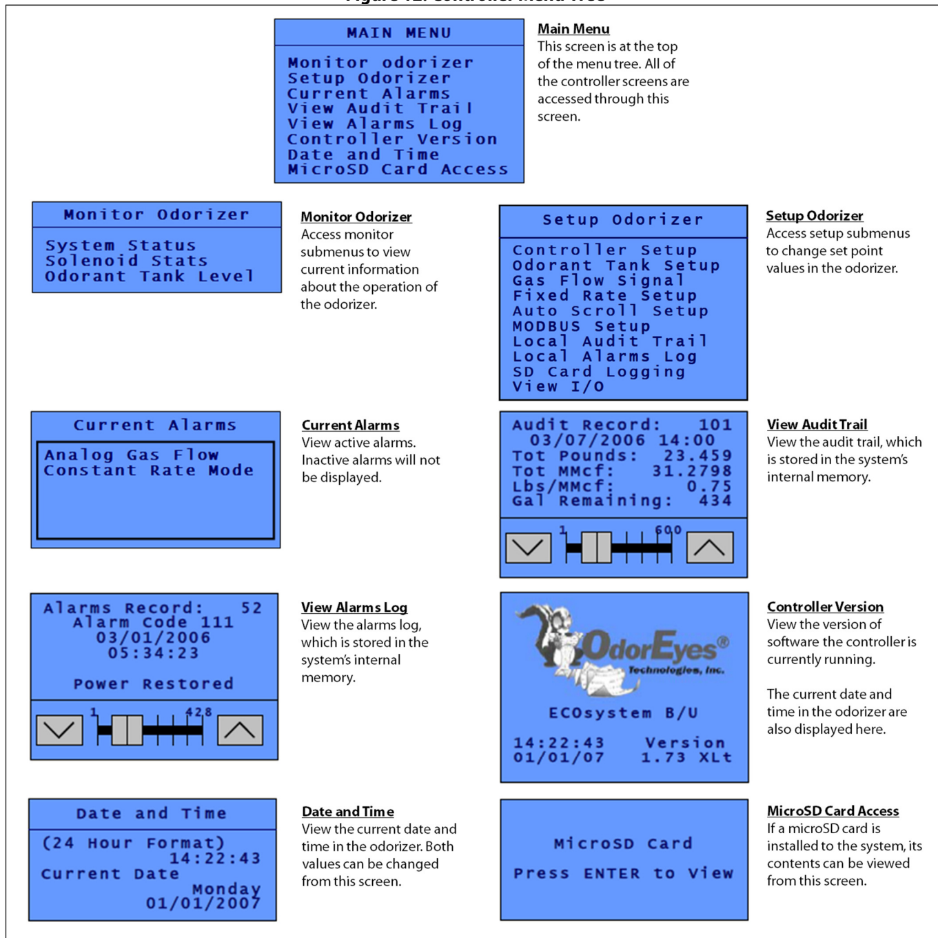
Figure 12: Controller Menu Tree
