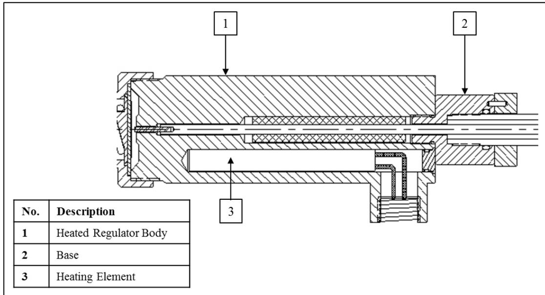
16. Remove the heated regulator body from the base and set it aside.
