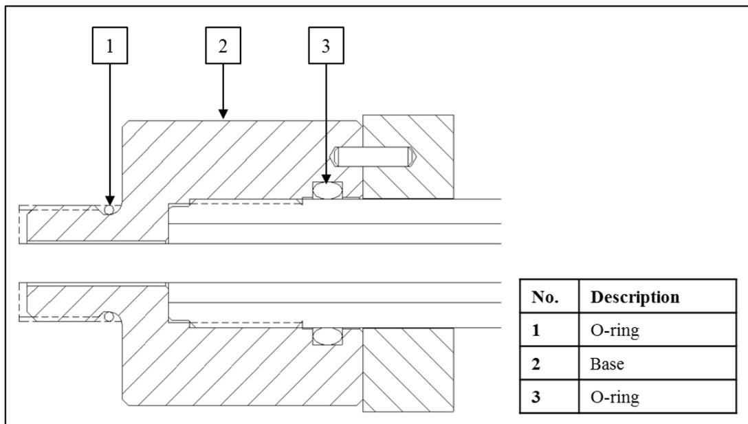
18. Reinstall the base to the heated regulator subassembly and tighten until there is no thread engagement.
