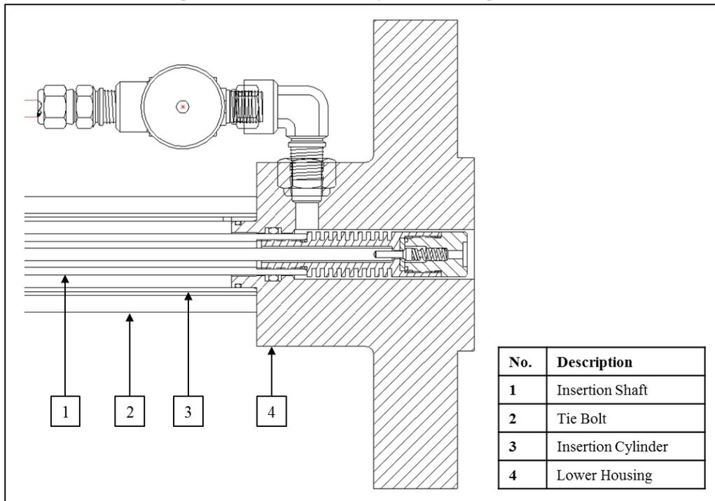
27. Replace the O-rings and back ups on the lower housing (*Figure 14*).
