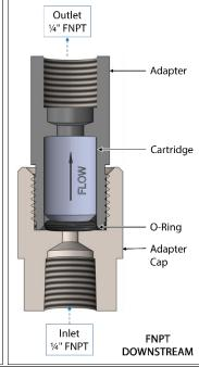
Figure 1: Welker® CV-K Check Valve Diagram
