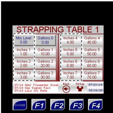
The left column of each table displays the tank depth in inches.
