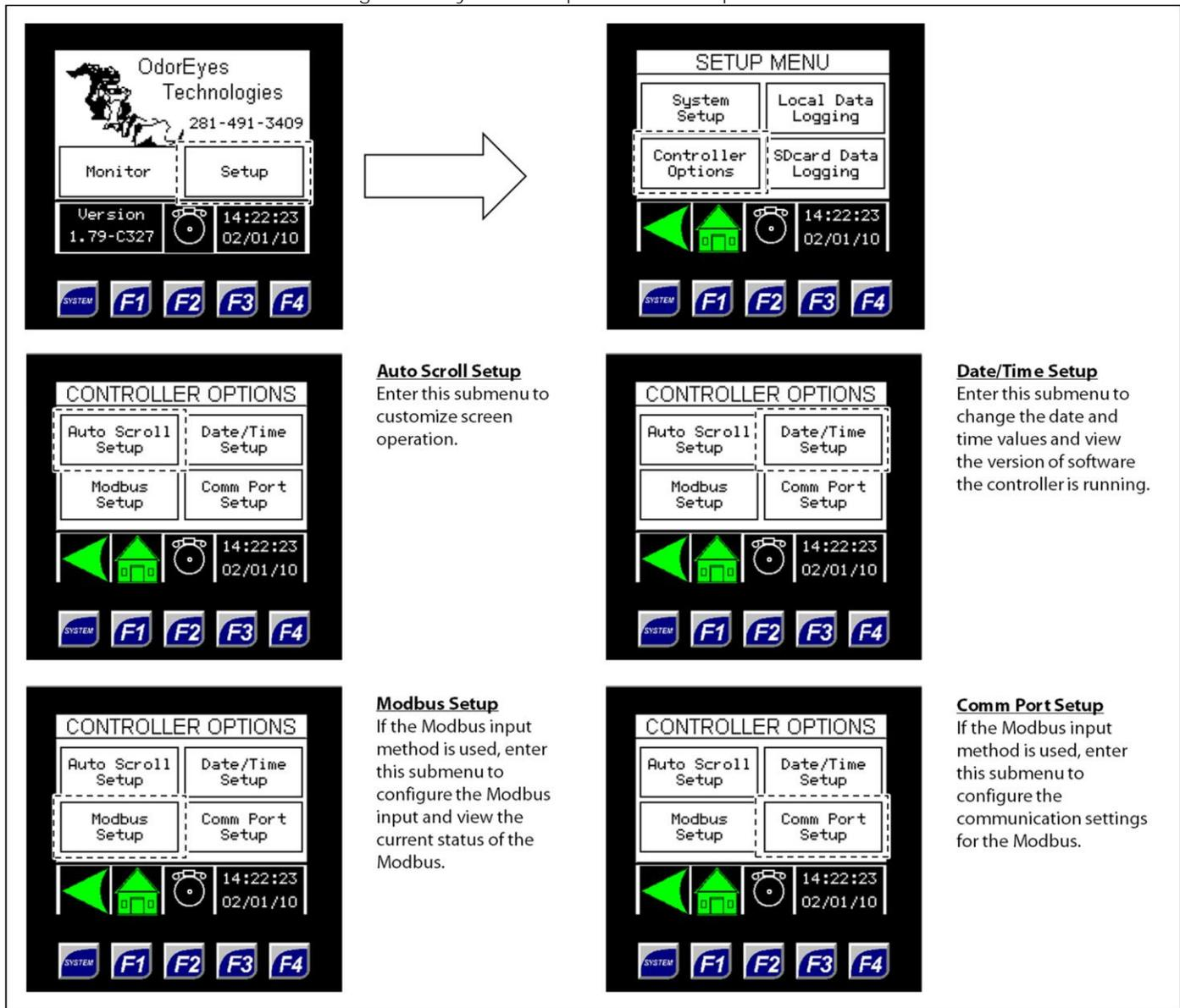
Figure 56: Controller Options – Auto Scroll Setup
