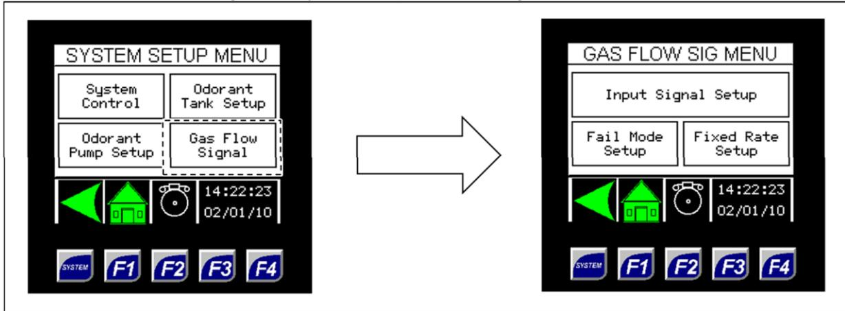
Figure 46: Gas Flow Signal – Input Signal Setup
