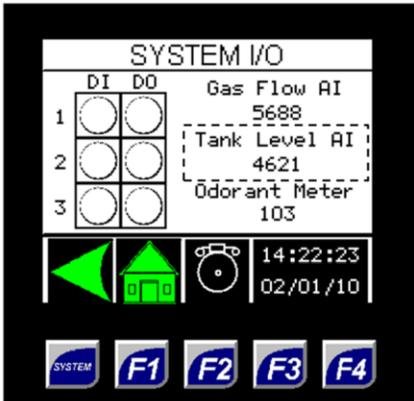
This analog signal is the raw count coming into the odorizer after the signal has been converted from milliamps. This value will vary according to customer specifications.
