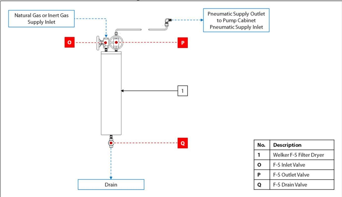
Figure 17: Optional Exhaust Filter
