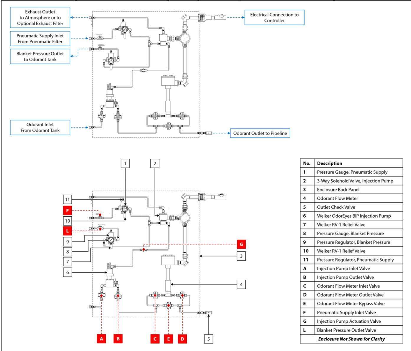
Figure 5: Pump Cabinet – Single SSO-9 Injection Pump With Blanket Pressure Regulator and Heater
