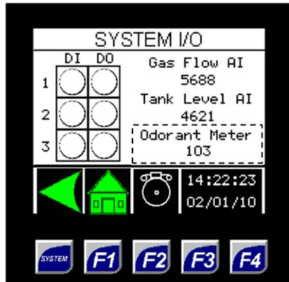
This value indicates how many high-speed pulses were received from the odorant flow meter. This value appears after each pump stroke and reverts to zero (0) after two (2) seconds.
