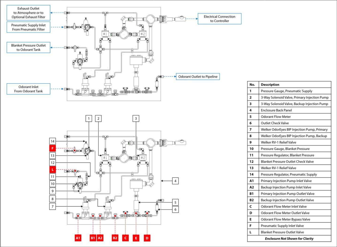
Figure 8: Pump Cabinet – Dual SSO-9 Injection Pumps With Blanket Pressure Regulator
