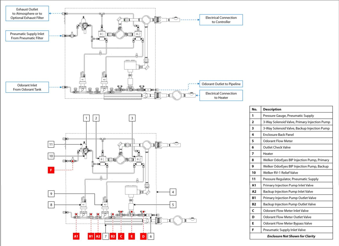
Figure 10: Pump Cabinet – Dual SSO-9 Injection Pumps With Blanket Pressure Regulator and Heater
