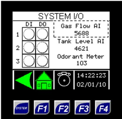
This analog signal is the raw count coming into the odorizer after the signal has been converted from milliamps. This value will vary according to the output from the customer gas flow meter.
