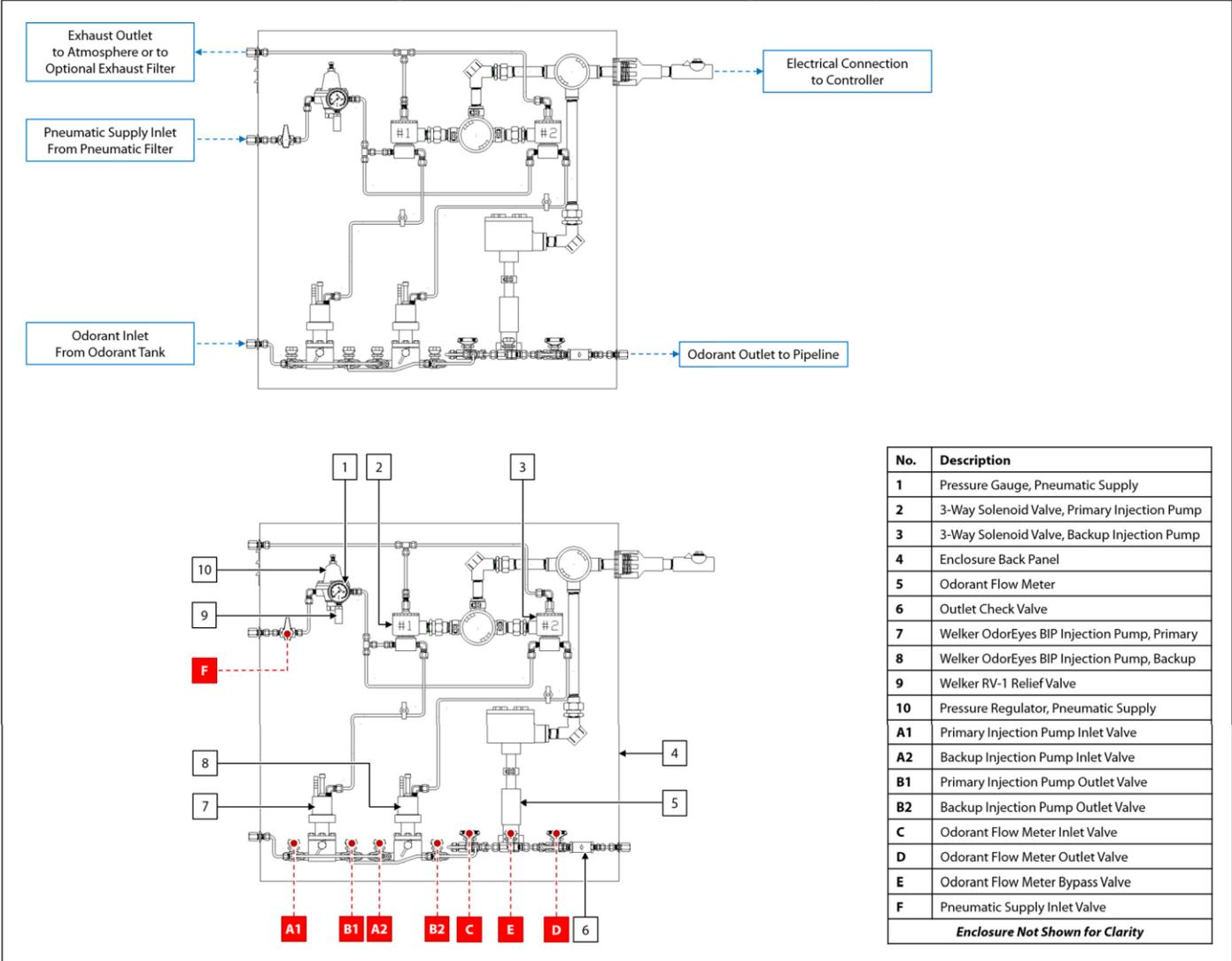
Figure 7: Pump Cabinet – Dual BIP Injection Pumps With Blanket Pressure Regulator
