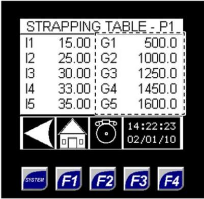
This column displays the tank volume in US gallons for five (5) strapping points.
