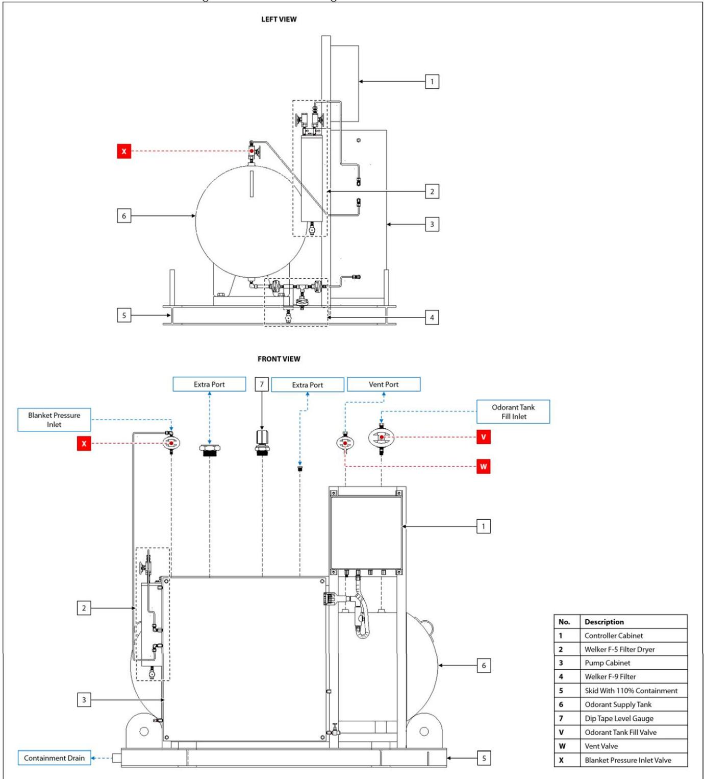
Figure 2: General Arrangement – Vertical Odorant Tank
