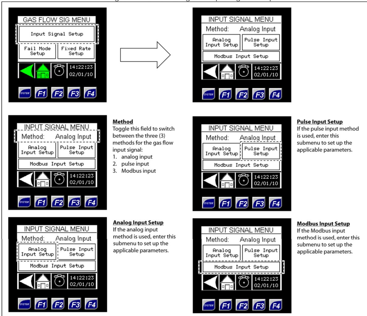
Figure 47: Gas Flow Signal – Analog Input Setup
