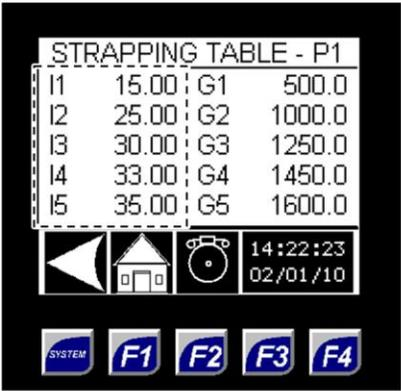
This column displays the tank depth in inches for five (5) strapping points.
