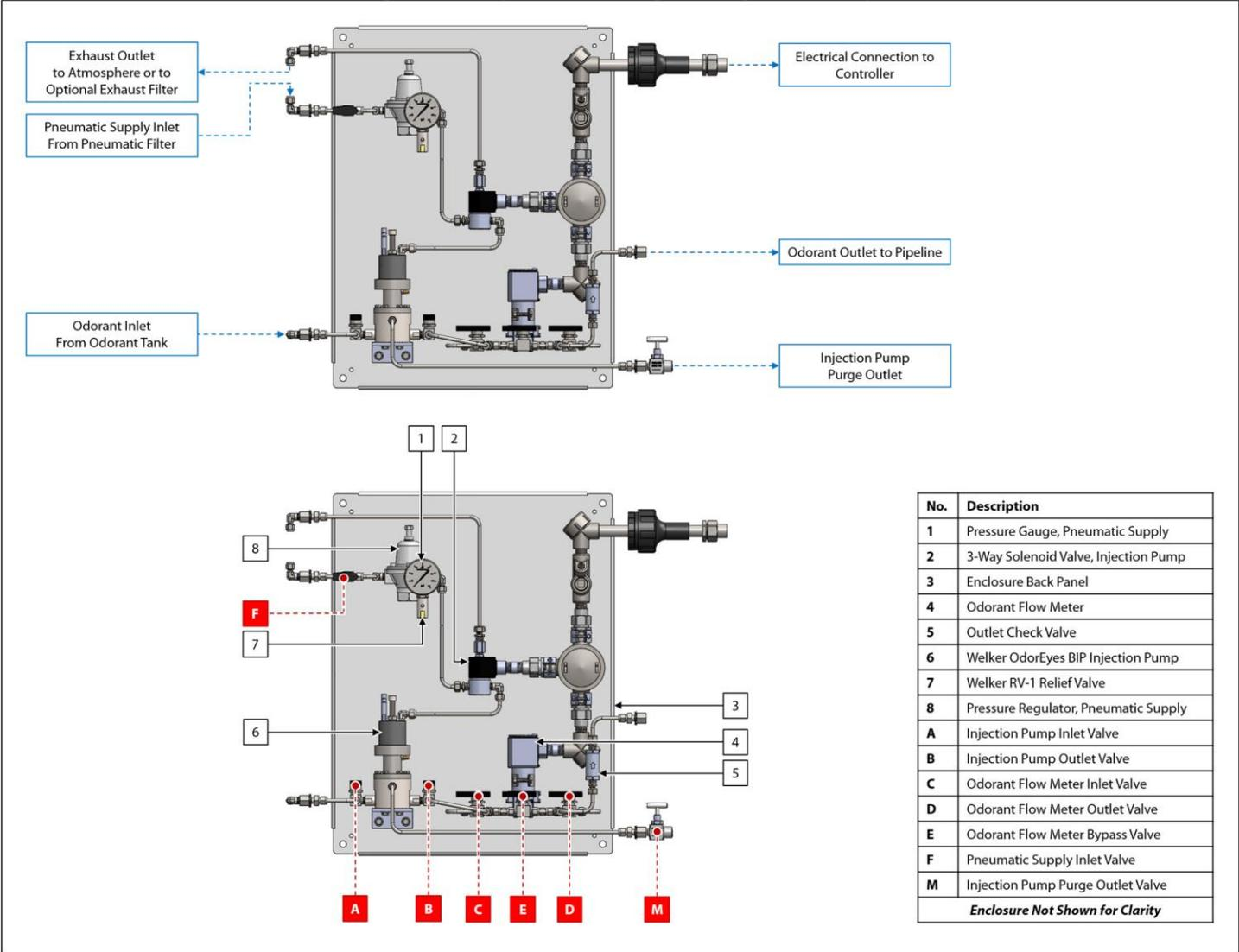
Figure 4: Pump Cabinet – Single BIP Injection Pump With Blanket Pressure Regulator
