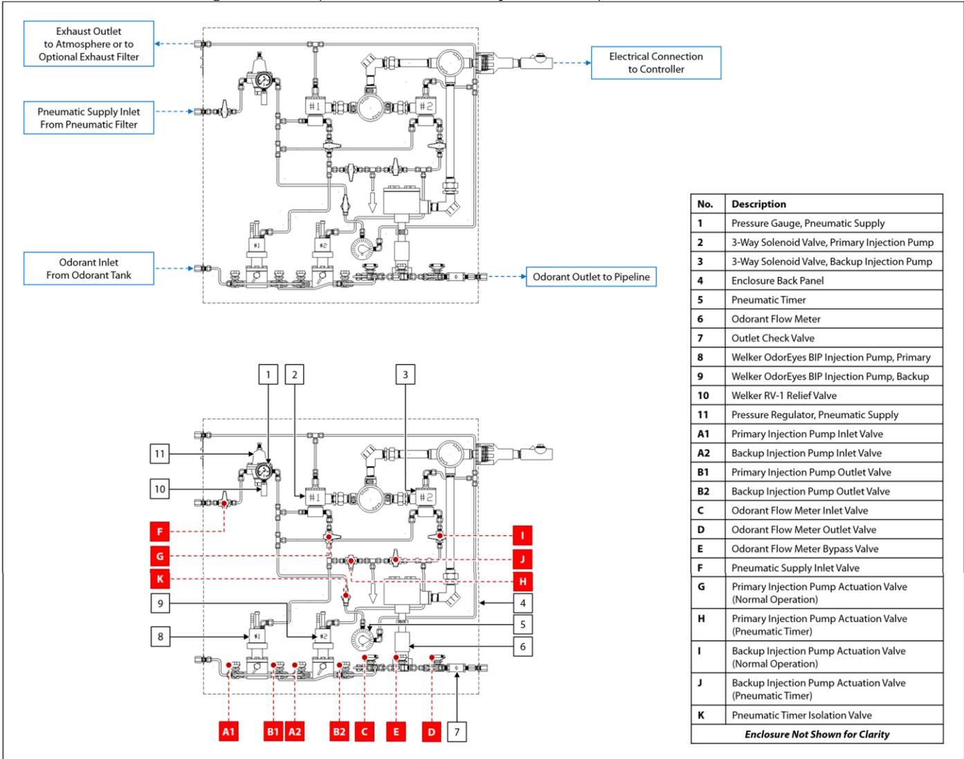
Figure 12: Pump Cabinet – Dual BIP Injection Pumps With Pneumatic Timer and Blanket Pressure Regulator
