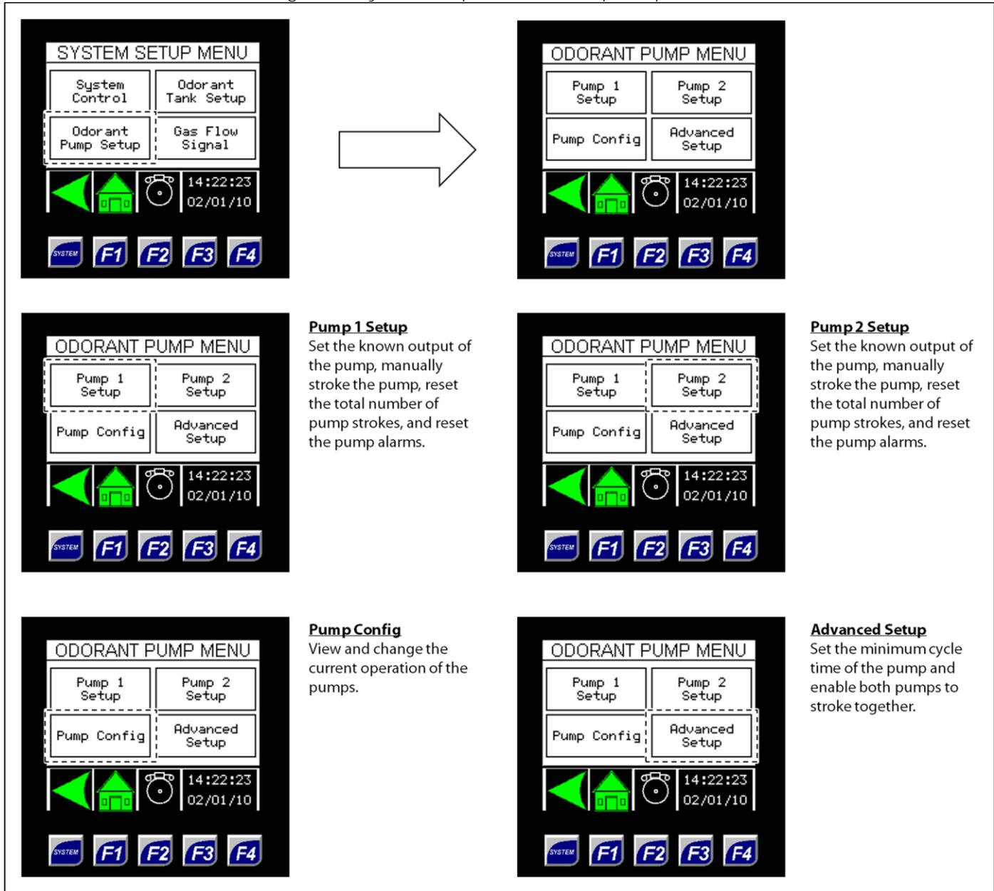
Figure 37: Odorant Pump Setup
