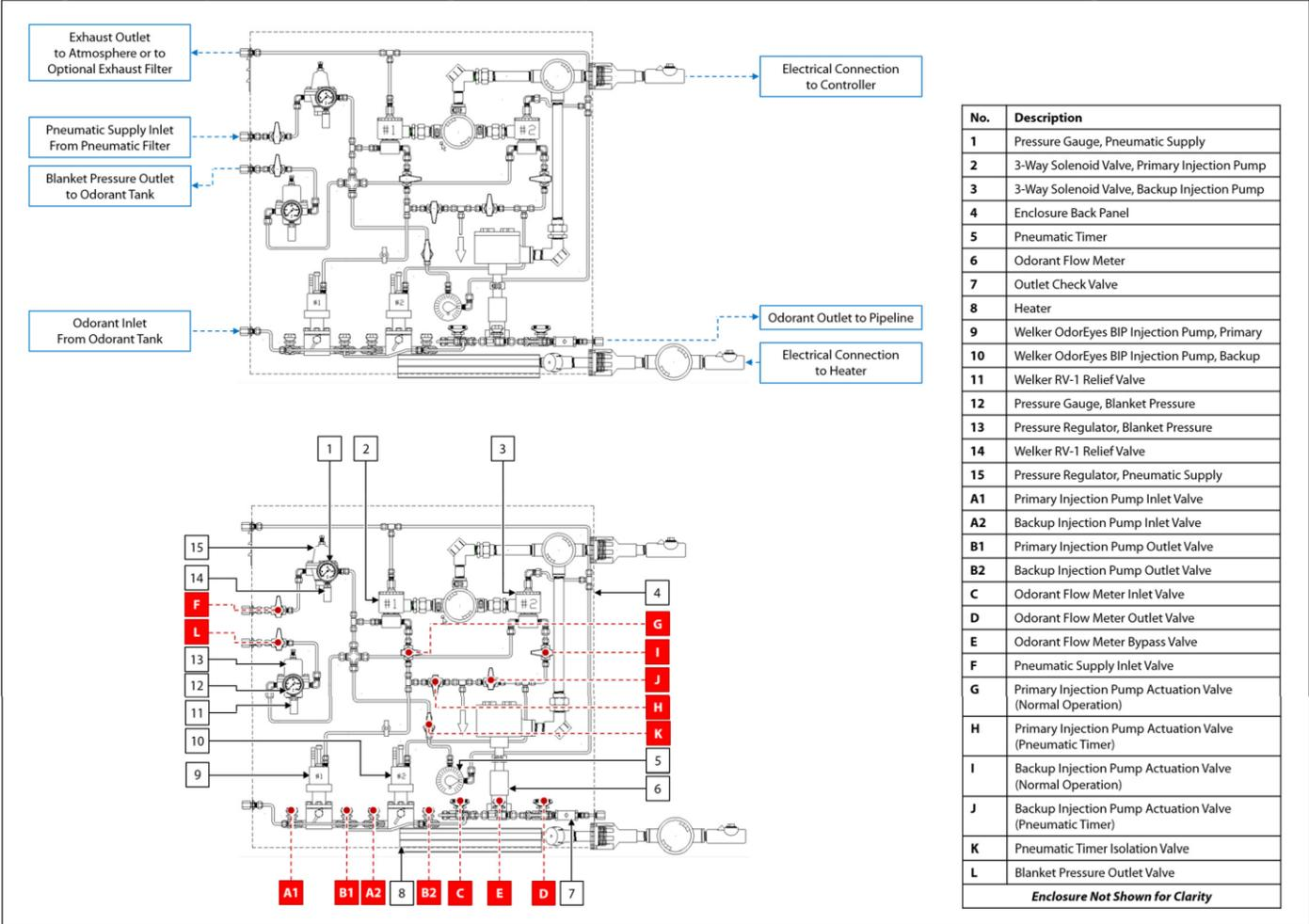
Figure 14: Pump Cabinet – Dual BIP Injection Pumps With Pneumatic Timer (No Flow Meter)
