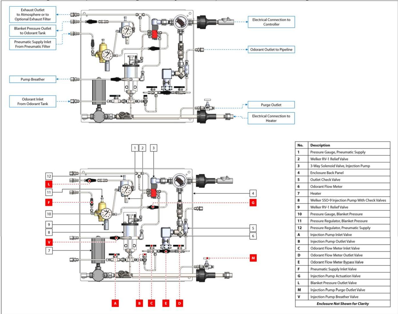
Figure 6: Pump Cabinet – Dual BIP Injection Pumps
