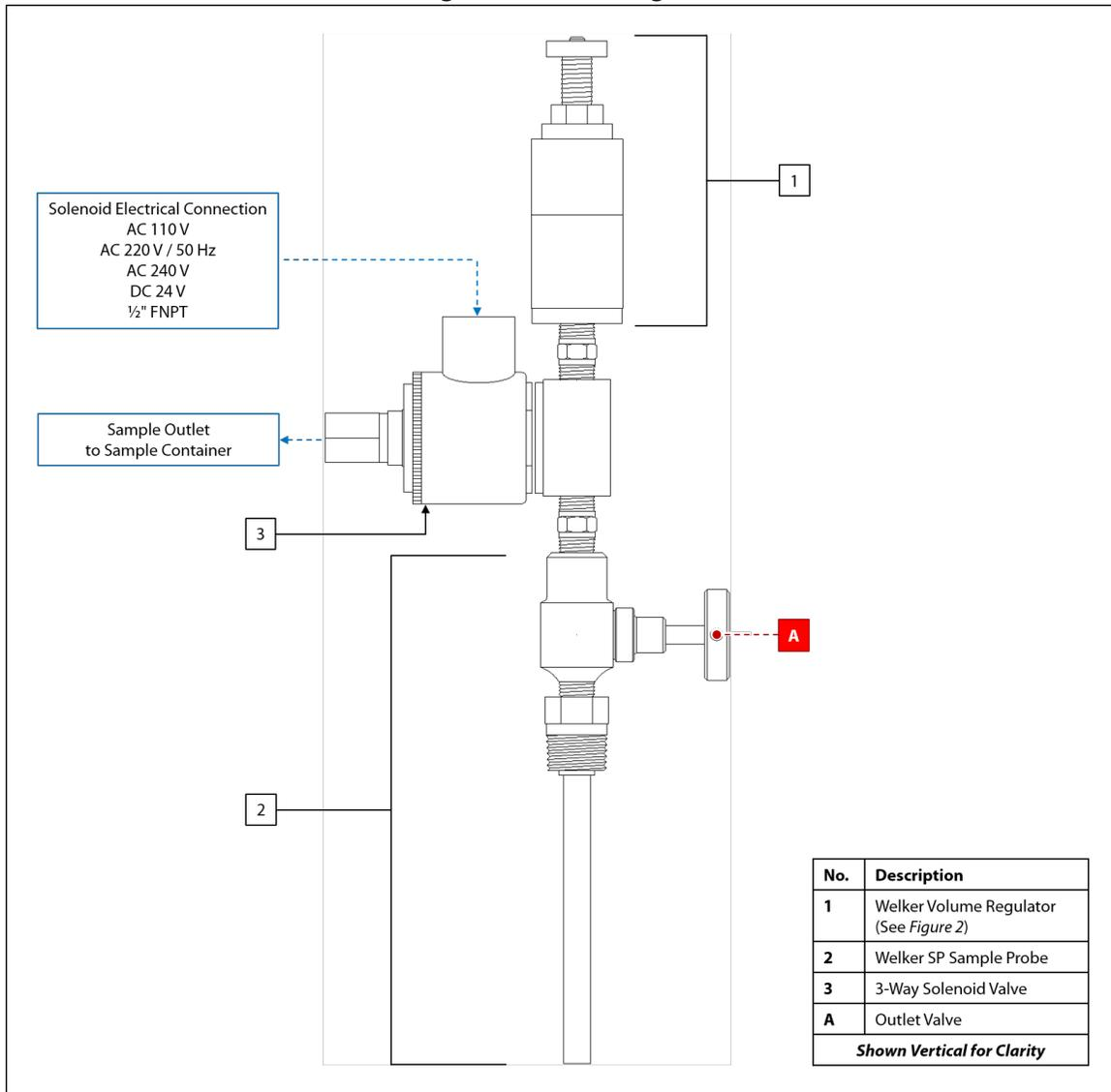
**Figure 2: Welker Volume Regulator Diagram**
