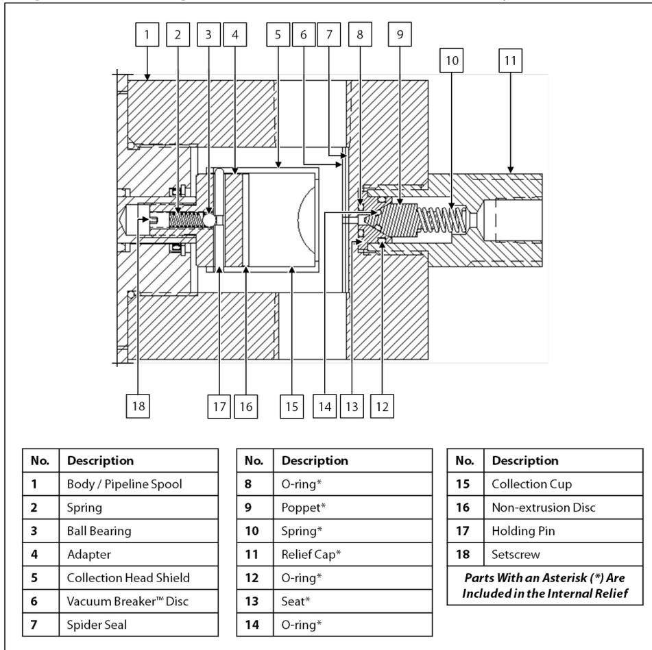
9. Unscrew the relief cap from the body / pipeline spool.
