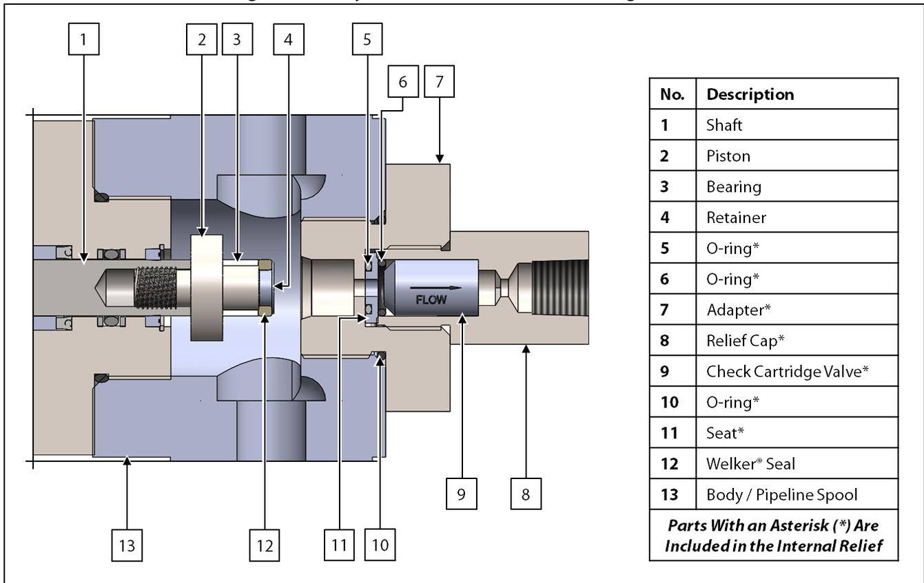
22. Unscrew the relief cap from the adapter.
