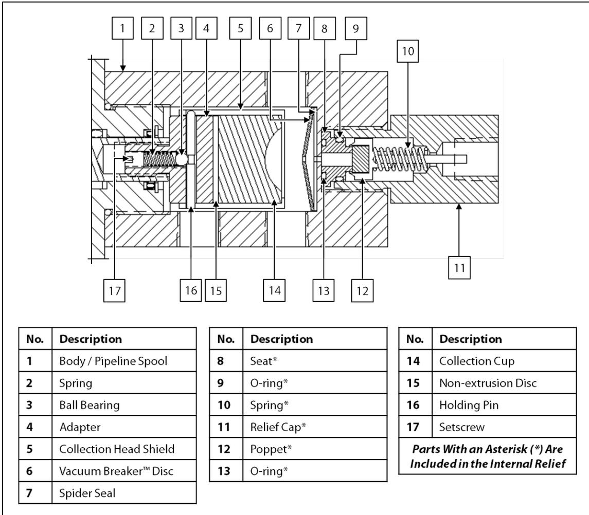
36. Unscrew the relief cap from the body / pipeline spool.
