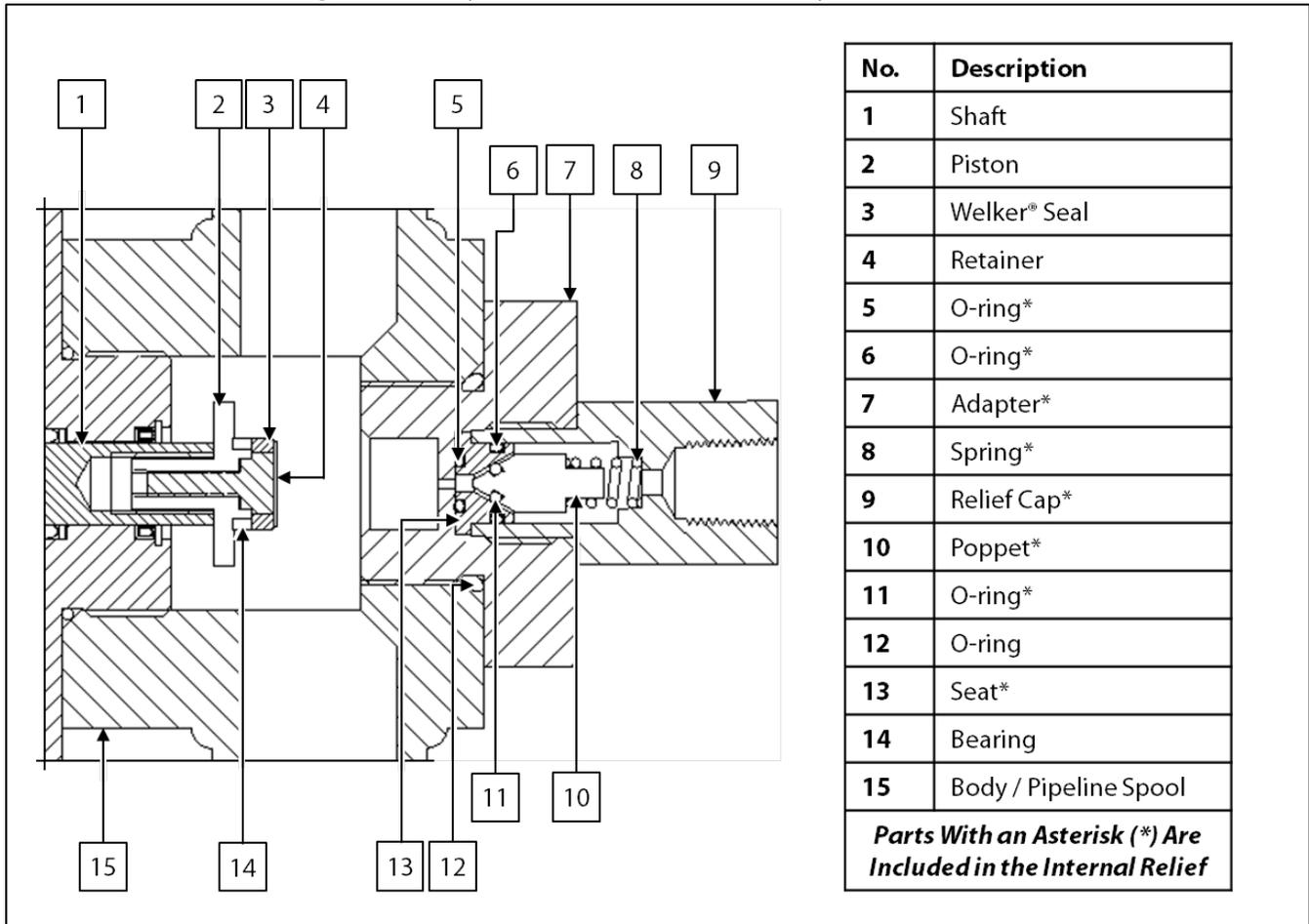
9. Unscrew the relief cap from the adapter.
