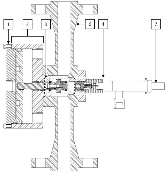
**PIPELINE SPOOL AND PACKING ADJUSTMENT NUT**
