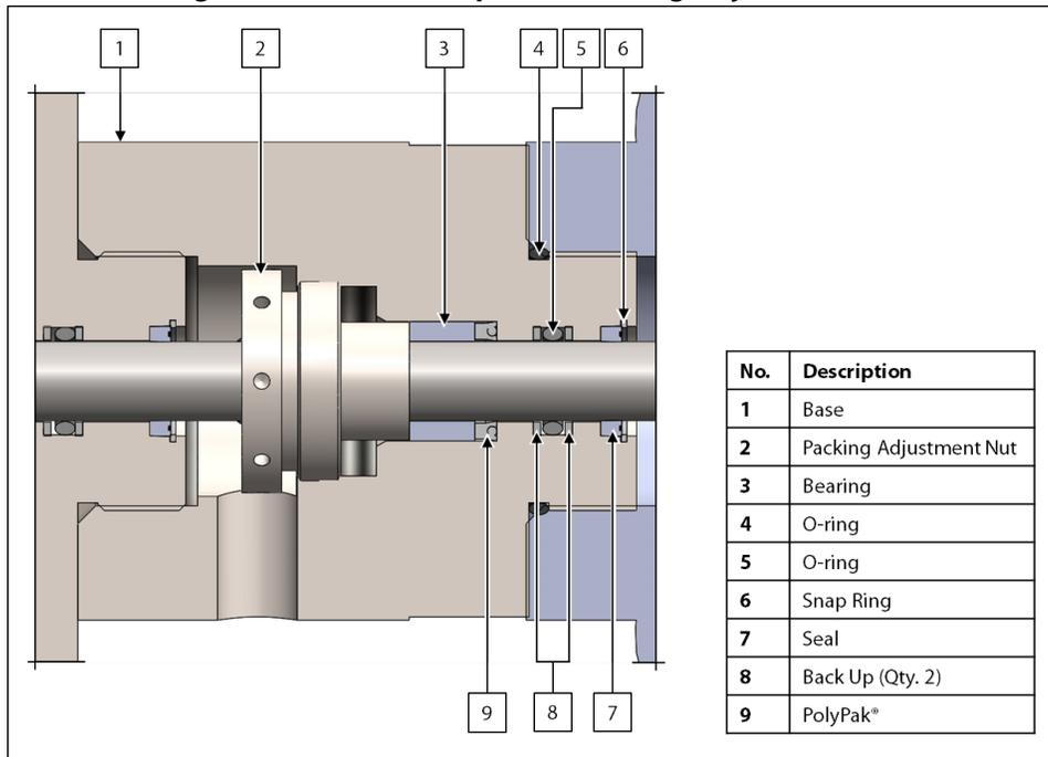
35. Unscrew the packing adjustment nut from the base.
