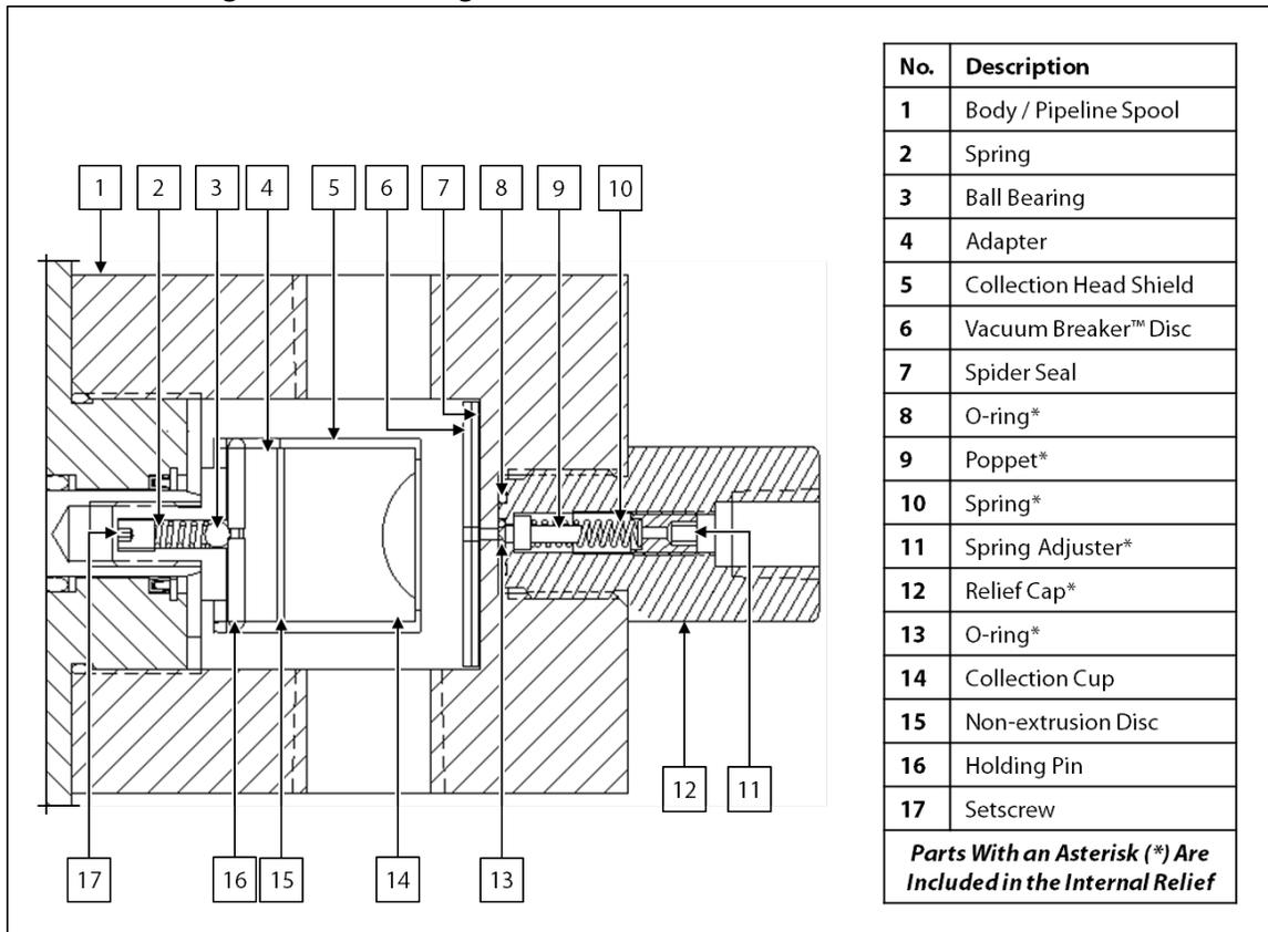
27. Unscrew the relief cap from the body / pipeline spool.
