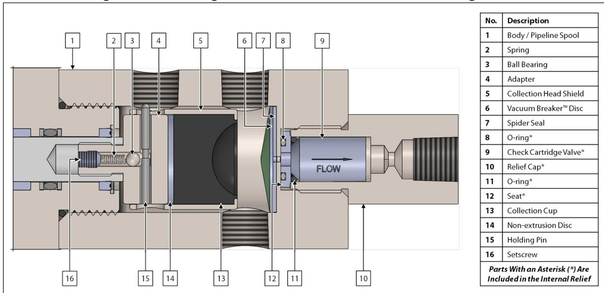
19. Unscrew the relief cap from the body / pipeline spool.
